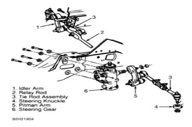
Fig. 7: Exploded View Of Steering Linkage (Express, G-Van & Savana) Courtesy of GENERAL MOTORS CORP.
