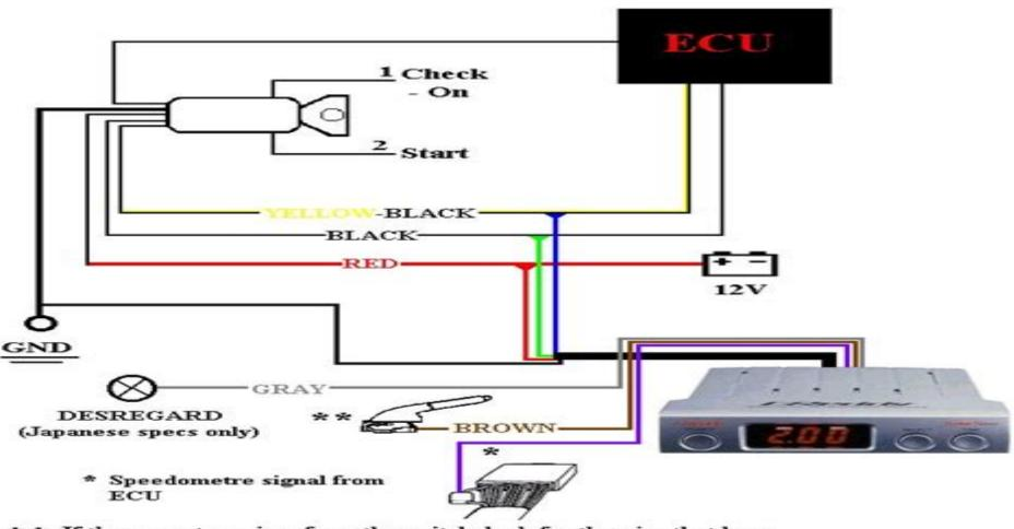
\*\* If there are two wires from the switch, look for the wire that has: 0V when parking brake is ON 12V when parking brake is OFF
