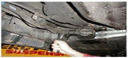
Step 1. Remove outer compensator arm bolt only. Remove two mounting bolts at cross pin, and parking brake cable retainer. At this time it is your discretion to remove complete trailing arm from vehicle to facilitate easier removal and installation of new polyurethane bushing or you may pull front of trailing arm downward.
