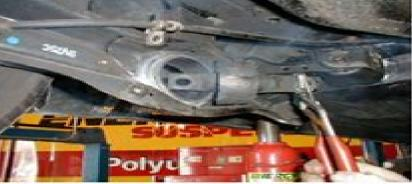
Step 2. Important Notes: Do not remove O.E. Outer metal shell. This shell is tapered on O.D.. Make note of which direction the cross pin is installed, this pin is offset! Bushing / pin removal. 1. Remove rubber bushing and / or pin from O.E. shell. (One example method to remove rubber bushing from O.E. shell is to use a hacksaw blade and cut bushing out. Note: All rubber must be removed from shell and clean for installation of new bushing.
