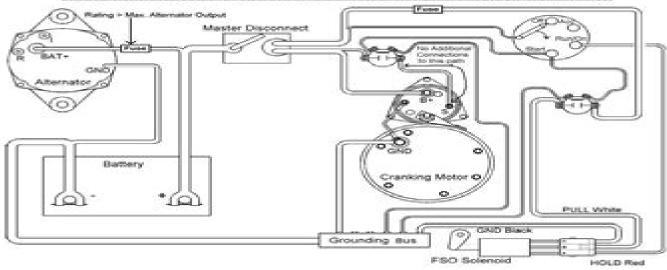
Figure 3.6 Low Current Fuel Shut-Off Solenoid (acceptable wiring method for current draw < 5 A)
