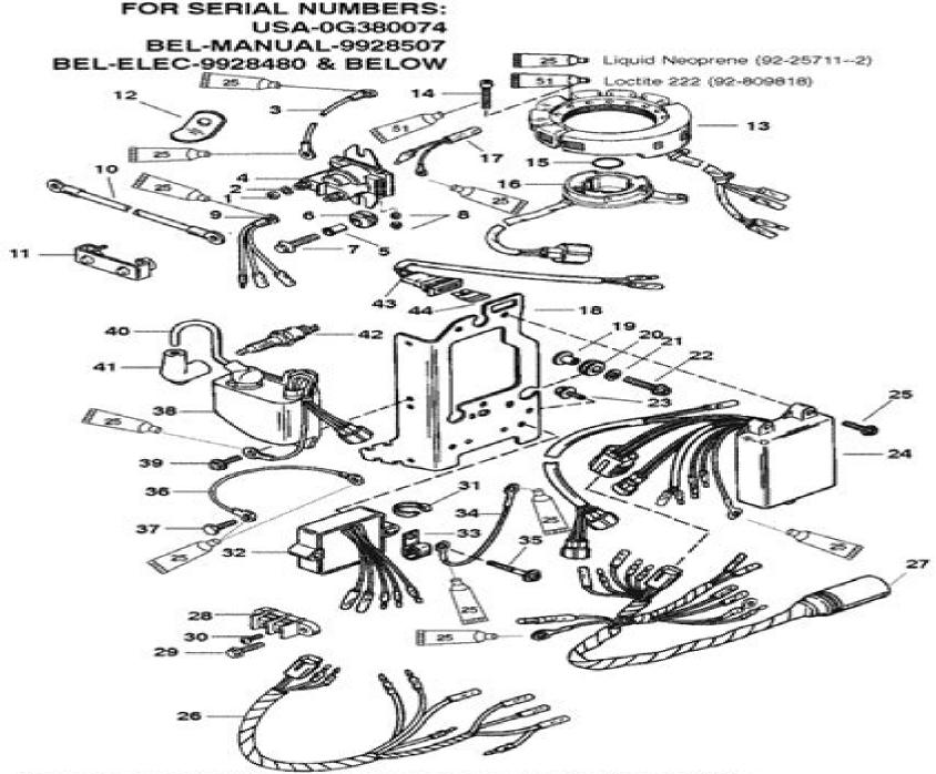
NOTE: APPLY LIQUID NEOPRENE TO ALL RING EYELET WIRING TERMINALS.
