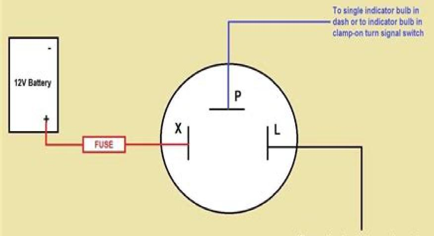
To turn signal switch power input wire
