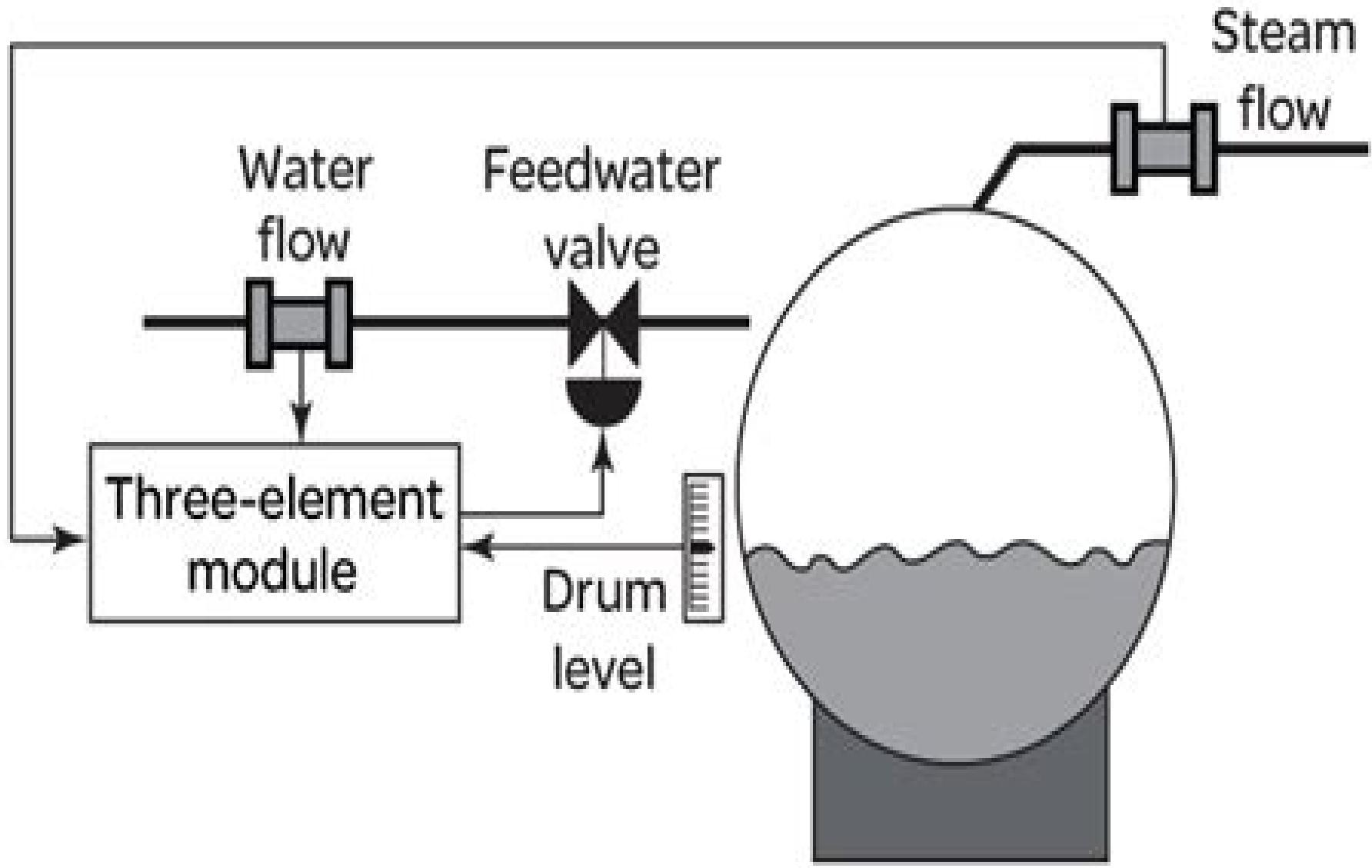
Figure 3 Three-element drum level control
