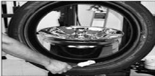
Figure 38 - Lubricate Tire Beads
