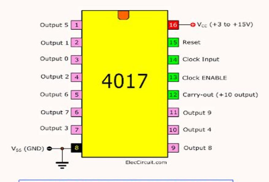
4017/CD4017 Pinout/ max voltage pin
