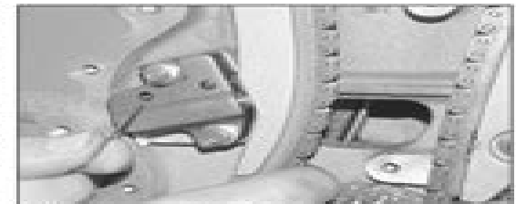
10.4 Press against the timing chain guide and insert a locking pin (approximately 1.5 mm)
