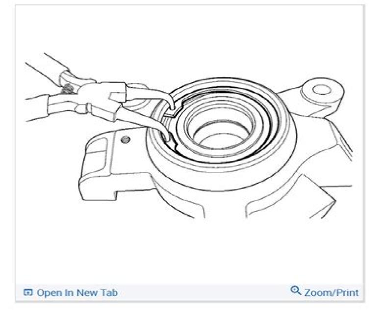
3. Install the wheel bearing retaining ring to the steering knuckle.
