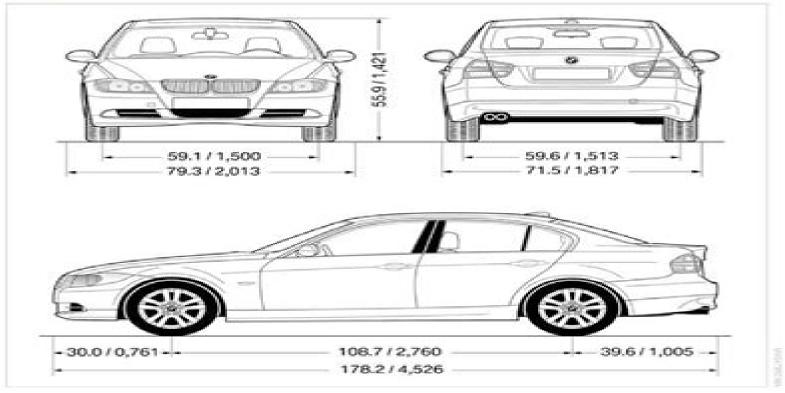
All dimensions given in inches/mm. Smallest turning circle diam.: 36 ft 1 in/11.0 m, with xDrive: 38 ft 9 in/11.8 m.
