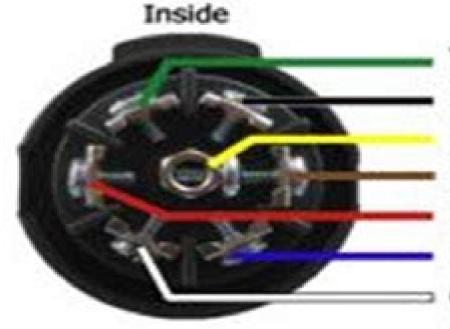
Tail & Running Lights 12V Power Reverse Lights Right Turn & Stop Left Turn & Stop Brake Controller Output Ground
