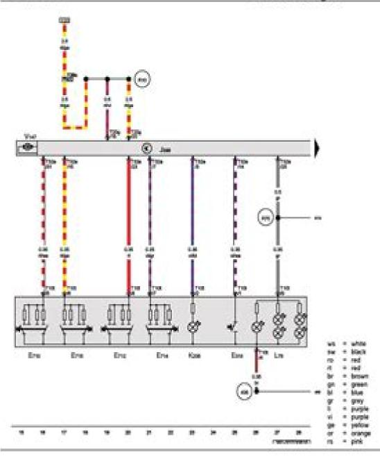
Front driver side window regulator button, Front passenger side window regulator button, in driver door, Driver door control unit, Driver side window regulator motor
