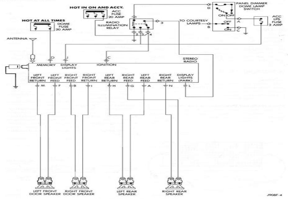
Fig. 3 Radio Schematic - SJ
