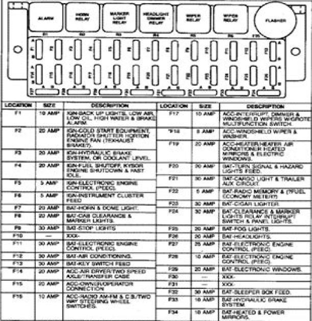
NOTE: LOCATIONS MARKED WITH AN " MUST USE A CIRCUIT BREAKER ONLY.
