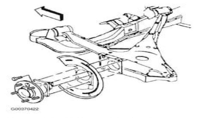
Fig. 1: Removing/Installing Wheel Bearing/Hub Retaining Bolts Courtesy of GENERAL MOTORS CORP.
