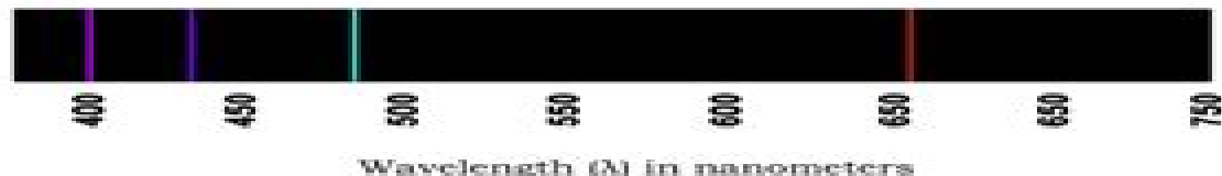
Figure1. Emission spectrum of hydrogen atom
