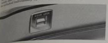
On the Piceturned Seventy-Five Lincousing the duce look switch is located on the left front door only. This excitch is provided on the right conv. An additional door look switch convenience of rear sout passengers. This switch will look and unlock all doors in the convenience manner.
