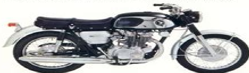
HONDA 450. A big bike with a big ride. Its OHC twin pumps out an astonishing 43 BHP @ 8,500 rpm, flies along at speeds up to 112 mph. Electric starting, exclusive torsion bar valve springs and low-end torque are bonus features.
