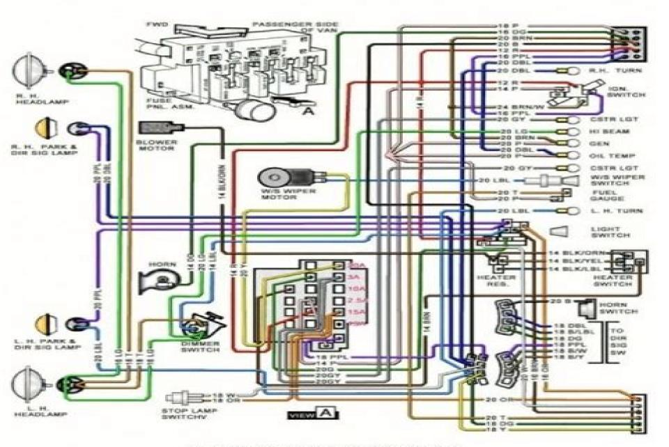
Fig. 43 - Front End & Instrument Panel (1966 Chevy Van)
