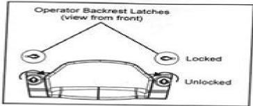
Tilt the backrest slightly forward towards the front of the vehicle and pull the passenger backrest upward from the bed of the cargo box.
