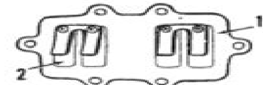
Fig. S24-4—View showing reed plate (1) and reed valve (2) assembly used on DT5 models.
