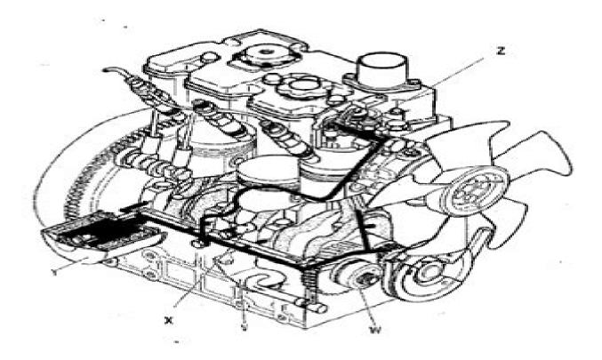
Suction filter Oil pump Relief valve Oil filter
