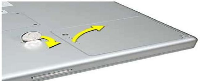
Touch a metal surface inside the battery bay to discharge static electricity built up on your body. (Figure 2)
