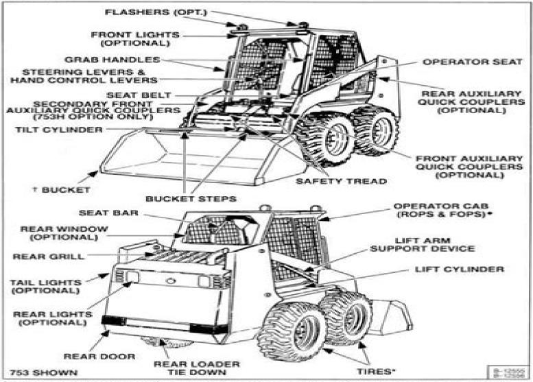
\* TIRES – Flotation tires are shown. The 753 Bobcat loader (shown) is factory equipped with standard tires. The 763 Bobcat loader is factory equipped with heavy duty flotation tires. See 753 & 763 Series Equipment for available optional tires.
