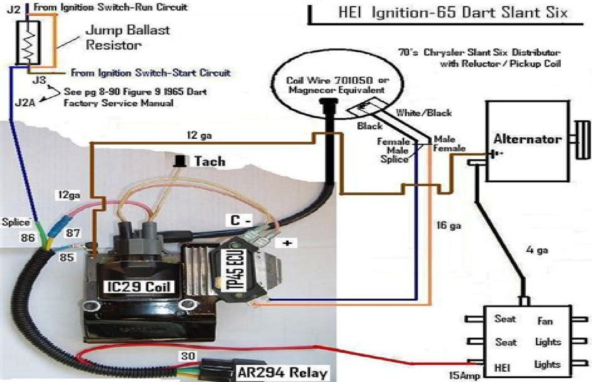
**Relay Harness EC23    Inner Fender Mounted Relay    Inner Fender Mounted Fuse Box**
