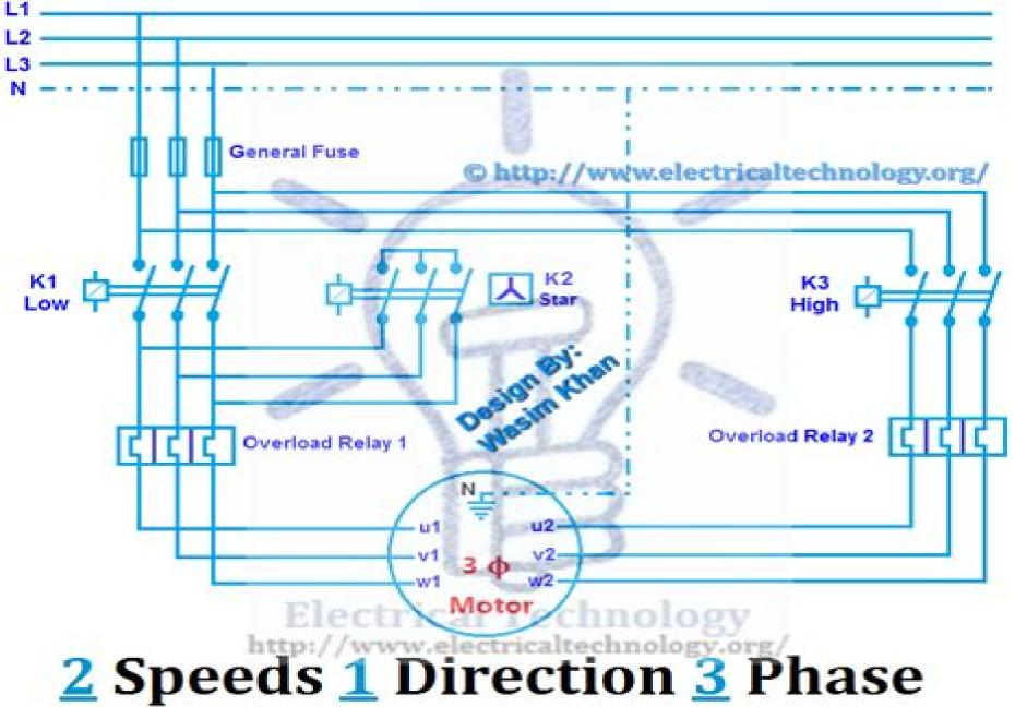
2 Speeds 1 Direction 3 Phase Motor Connection Power Diagram
