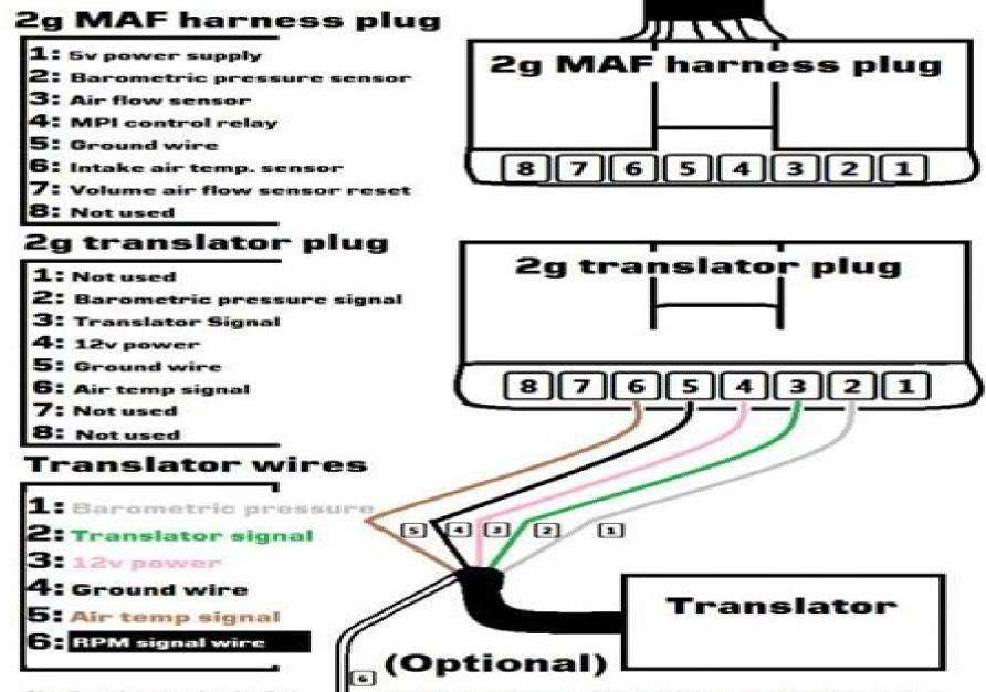
Also there is a purple wire that is used for nitrous or alchohol injection. If not using just loop inside translator box. The RPM signal wire(white) from the translator needs to be connected to a TACH signal. You can get a signal from the power transistor pin #5 or from ECU pin #58.
