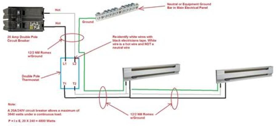
4500 watts/1.25 + 3840 watts maximum on a 20 amp circuit
