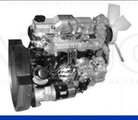
In-Line 4 Cylinders / OHV / Diesel
