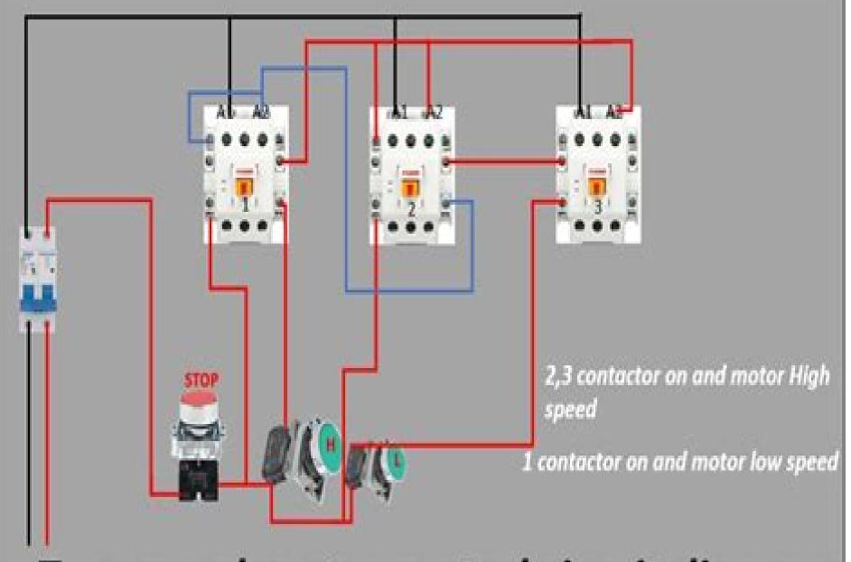
Two speed motor control circuit diagram
