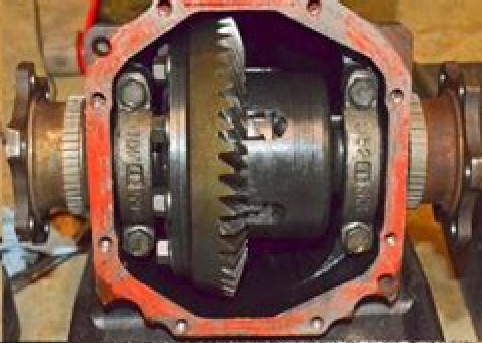
This one is out of an Auto 350Z/G35 and has the 3.357:1 Gear Ratio. It has a Cusco RS LSD in it. Note the Ring gear is thicker and the mounting surface on the Diff. is off to the left compared to that of the one that came out of a Manual 6 Speed.
