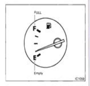
The gauge indicates the APPROXIMATE fuel level in the tank.
