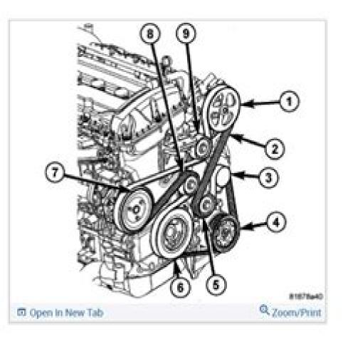
NOTE: When installing drive belt on the pulleys, make sure that belt is properly routed and all V-grooves make proper contact with pulley grooves.
