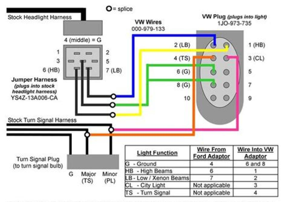
Remember to upgrade the fuses (change Fuses #16 & #17 from 10A to 15A), and install a jumper wire on pins #8 and #9 of the multifunction turn signal switch).
