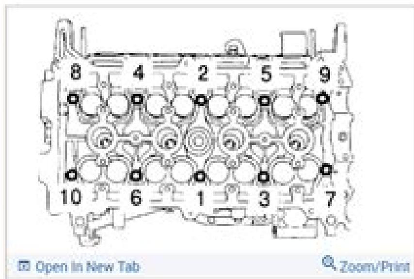
b. Using a 8 mm bi-hexagon wrench, install and uniformly tighten the 10 cylinder head bolts and plate washers, in several passes, in the sequence shown.
