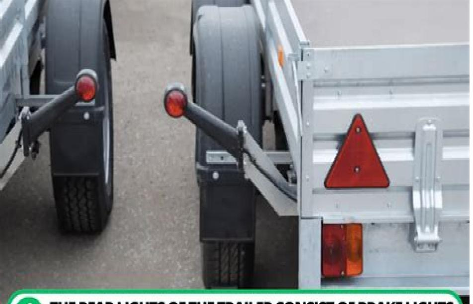
THE REAR LIGHTS OF THE TRAILER CONSIST OF BRAKE LIGHTS, TAIL LIGHTS, NUMBER PLATE LIGHTS AND TURN SIGNALS
