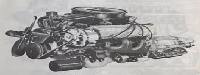
View of 4146 cc. (253 cu in.) Engine Assembly.
