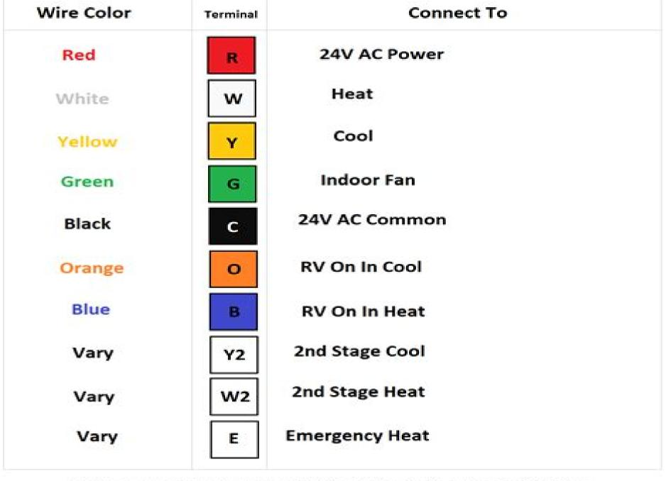
Color Code and Terminal for Heat Pump Thermostat Wiring
