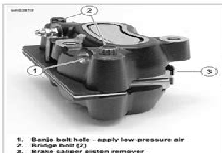
Figure 2-36. Removing Pistons
