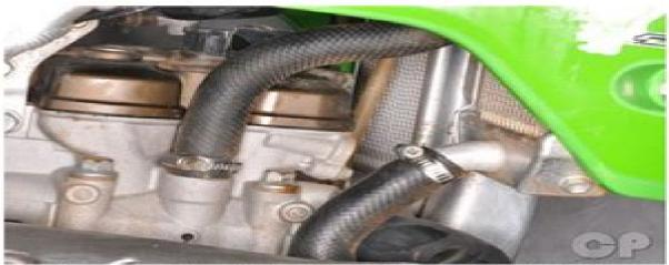
Inspect the coolant hoses for damage and deterioration. Replace hoses as needed. Make sure the connections are secure and not leaking.
