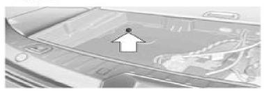
Forcefully pull the release tool up against the resistance until you notice a marked increase in the resistance and the parking brake releases audibly.
