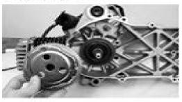
Remove the washes and peedle bearing.
