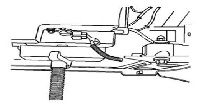
Fig. 4: View Of Wood Block Between Engine Oil Pan & Pole Jack Courtesy of GENERAL MOTORS CORP.
