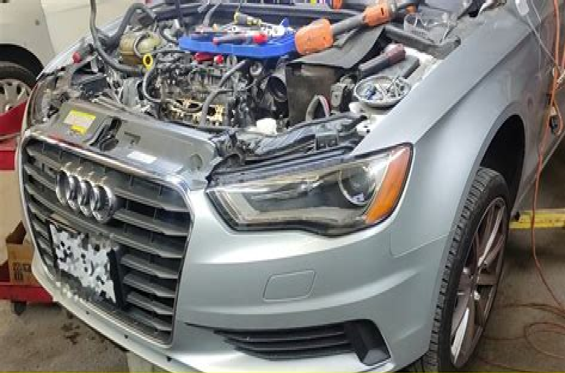
2015 Audi A3 Radiator Removal No Bumper Removal
