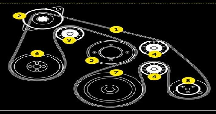
1 BELT 2 ALTERNATOR 3 A BELT TENSIONER 4 IDLER PULLEY 5 WATER PUMP 6 POWER STEERING PUMP 7 CRANKSHAFT 6 AIR CONDITIONING COMPRESSOR
