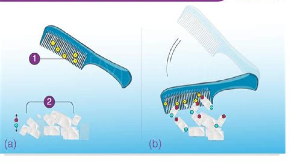
(b) The comb attracting small pieces of paper with static electricity.
