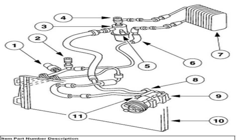
1 19D594 A/C Pressure Cut-Off Switch
