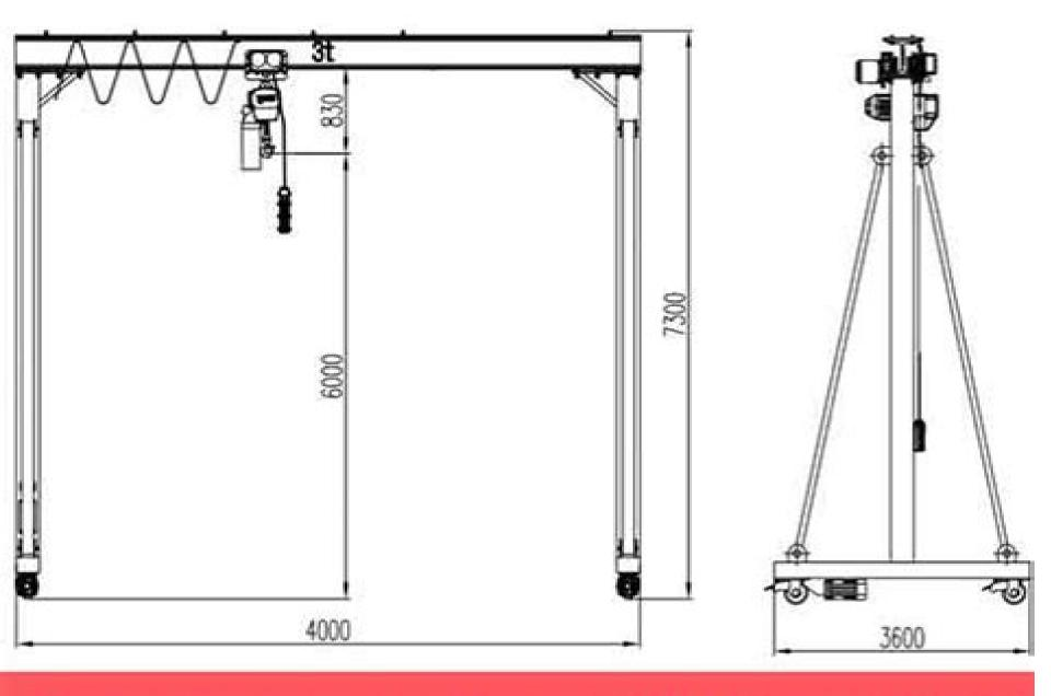
3 ton Portable Gantry Crane WWW.EOTCRANEKIT.COM
